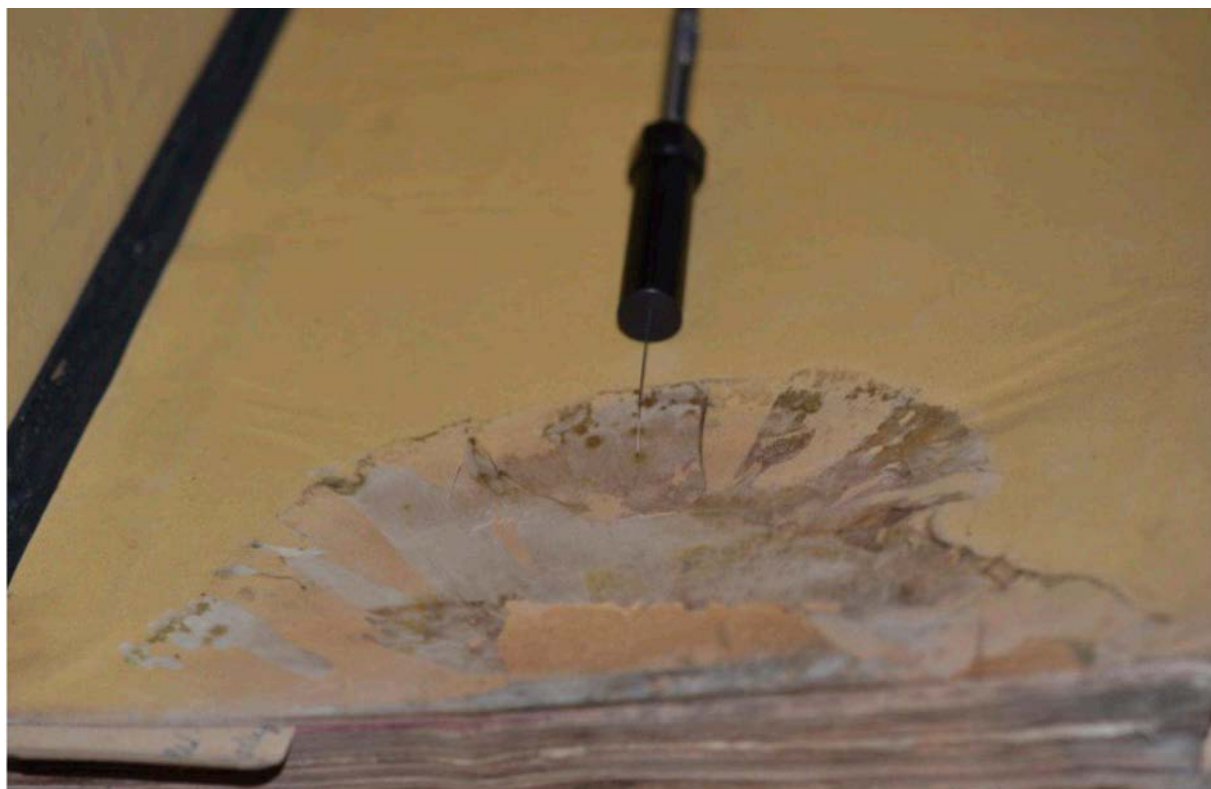
Figure 1: Sampling of MVOCs on SPME fibre in a 19 th century book with a visible alteration on the surface of the first page, which suggests the presence of the active mould.
